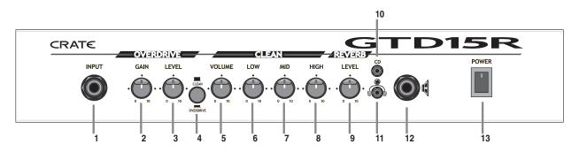
**1. INPUT:** Use this jack to connect your guitar to the amplifier by means of a shielded instrument cable.
